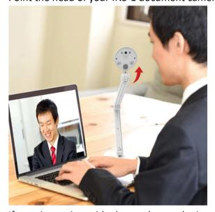
4. If your image is upside down, change the image orientation by simultaneously pressing both the brightness(+) and the brightness(-) buttons.
